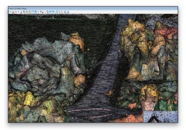
OpenRoads Designer includes reality modeling tools to incorporate and edit all reality modeling data types, including the capability to extract ground-level features from reality meshes and LiDAR, as well as to reference point clouds and imagery.
