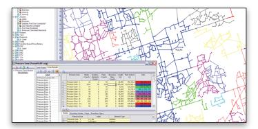
The Pressure Zone Manager automates the process of identifying the multiple pressure zones of a water distribution system and their characteristics.
